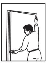
Usually, it is only necessary to adjust the top hinge. However, if there is still a large gap between the
