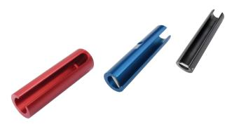
**INSTRUCTIONS:** This tool is designed to adjust new, worn, or improperly adjusted commercial butt hinges that cause the door to sag or drag. To fix the door, slip the tool over the top door hinge, and open the door. This action causes the door hinge to bind while the tool is in place.
