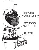
Install battery compartment cover and secure with retaining screw. Make certain that battery compartment cover is fully compressed against gasket to provide a seal. Do not overtighten. Plug the electrical connector into the battery compartment cover. Reinstall the sensor module onto the plate. Reinstall the complete cover assembly onto the plate. Tighten the two (2) screws on top of the unit.
